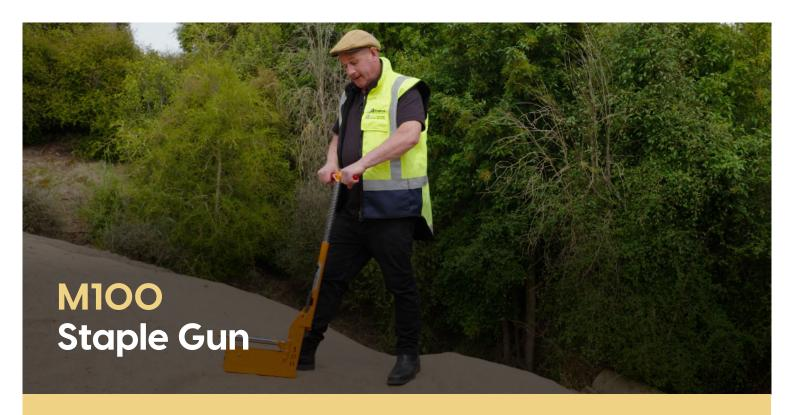
Made in Canada, the M100 staple gun uses 150mm staples and will increase productivity and reduce labour costs when installing erosion control blankets, geotextiles and landscape fabrics.
